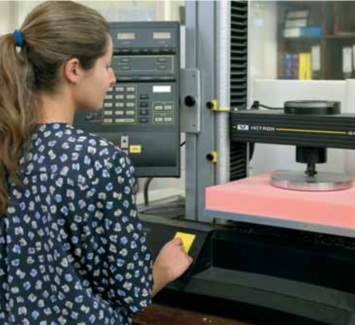
All Joyce foam is tested to ensure it conforms to AS2281 for density and hardness.
